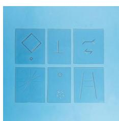
Set of 6 examples to demonstrate optical and haptic illusions, transparent polystyrene, for use with the overhead projector
